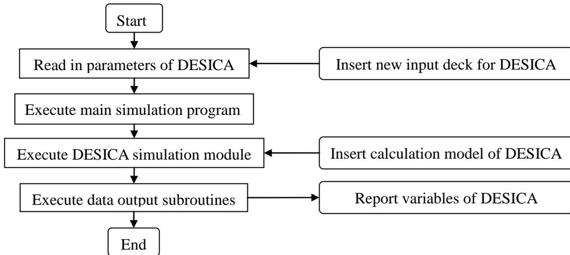
**Figure 2.** Schematic flowchart of the compiling process of DESICA system
