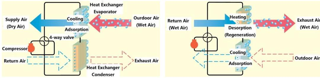
**Figure 1.** Schematic diagram of DESICA
