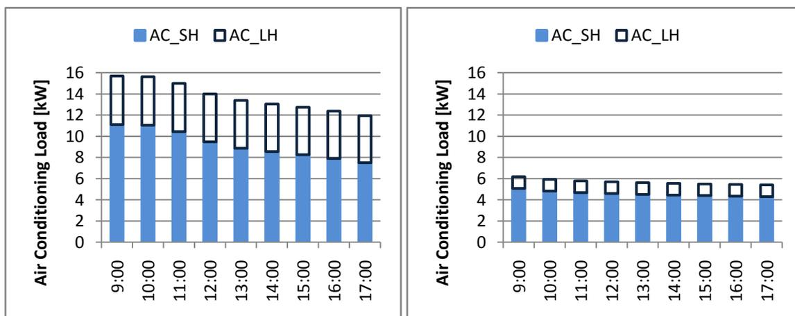
**Figure 4.** Air conditioning load on typical design day: summer and winter
