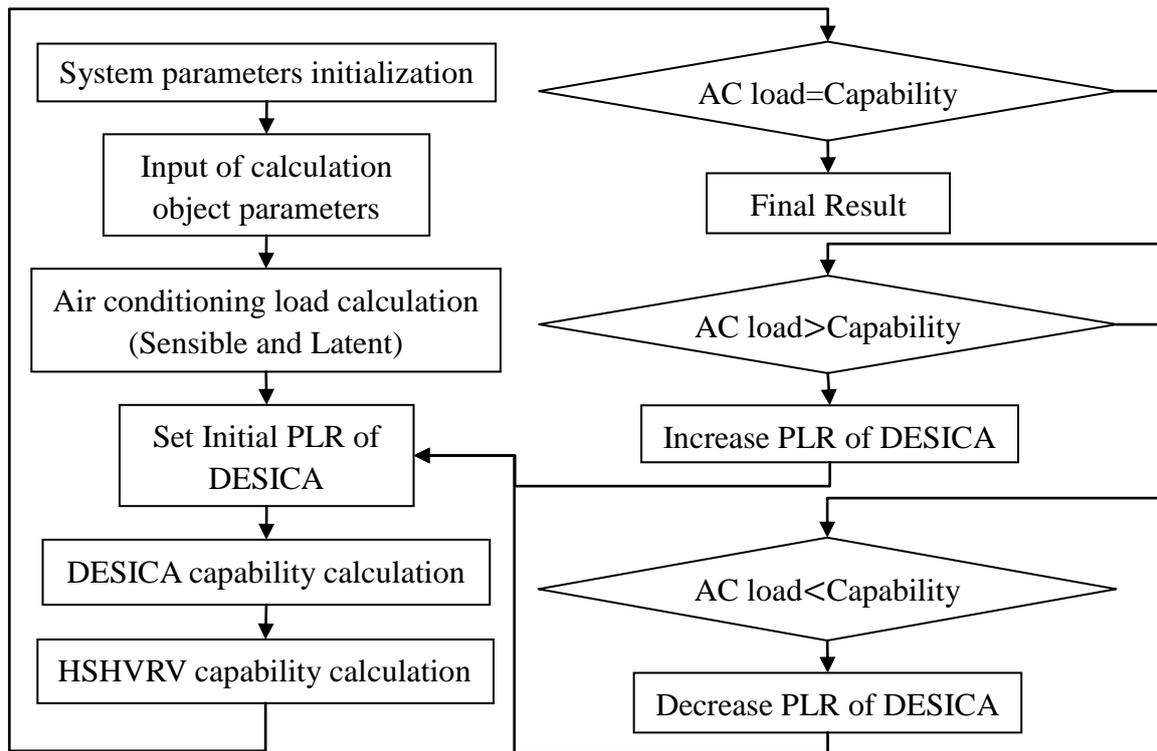
**Figure 3.** Schematic flowchart of the calculation program for JDHVS
