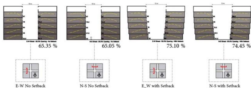
**Figure 7.** Parametric daylight availability study
