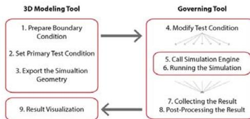
**Figure 1.** Proposed simulation workflow
