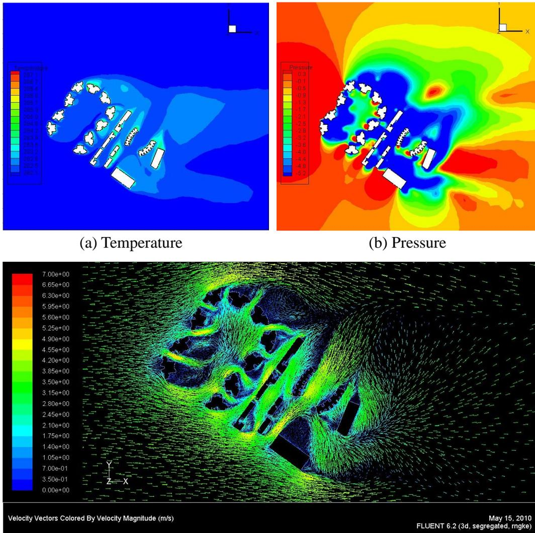
**Figure 4.** Simulation results of wind environment in winter
