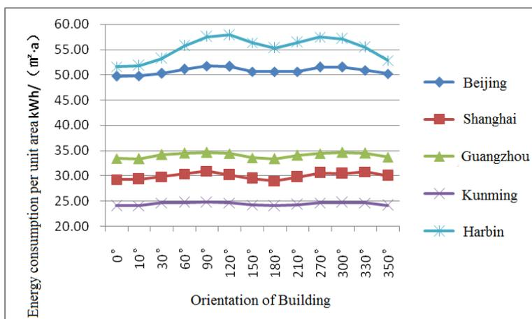
There is an obvious difference should be noticed: the optimal orientation of buildings in Harbin, Beijing and Shanghai is between the south by east 5°-15°, which conforms to our common sense, but the optimal orientation of Kunming and Guangzhou buildings is between ±5° of north, which conflicts our experience.
