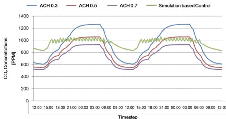
**Figure 6.** CO<sub>2</sub> concentrations with simulation based control and constant ventilation rates
