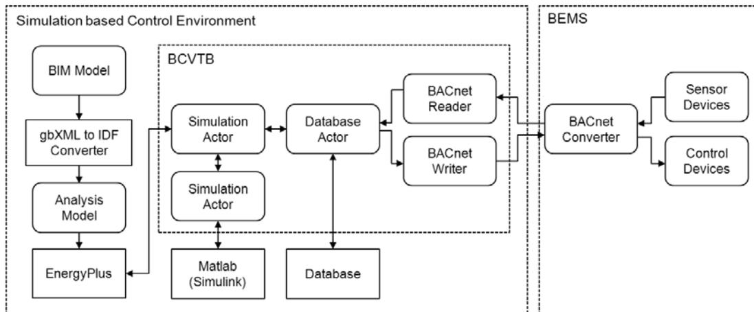
**Figure 1.** A framework of a simulation-based control system in the operational stages
