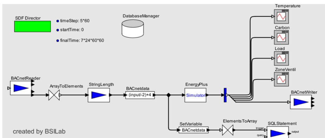
**Figure 4.** Ptolemy II model for the integrated simulation based control in the BCVTB
