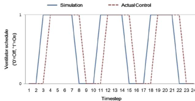
**Figure 5.** Simulated ventilator schedule using EMS and actual operation schedule for ERV
