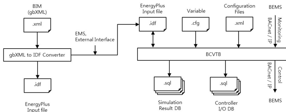
**Figure 2.** Input/output data required for the simulation-based control system
