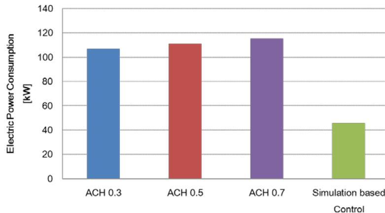
*Figure 7. Electric power consumptions from ERV*
