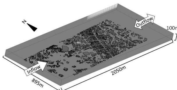
**Figure 4. 3D model for CFD simulation**
