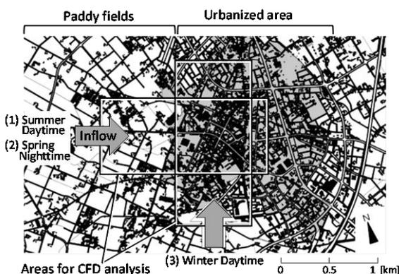
**Figure 3.** Subject area for the microclimate analysis using CFD simulation (including the field measurement points)
