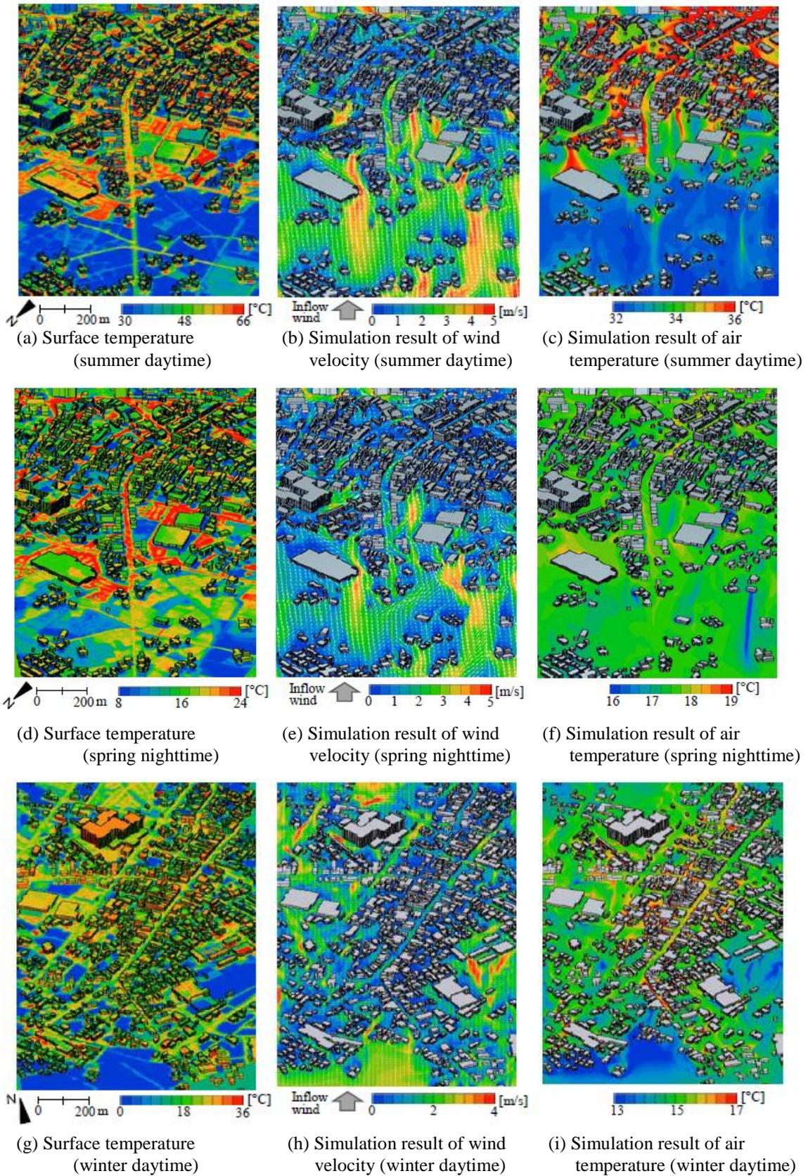
**Figure 6.** 3D surface temperature images, CFD simulation results of wind velocity and air temperature distribution for each case
