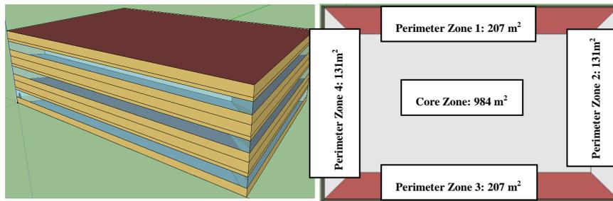
**Figure 1.** Medium office building (left) and thermal zones of a typical floor (right)
