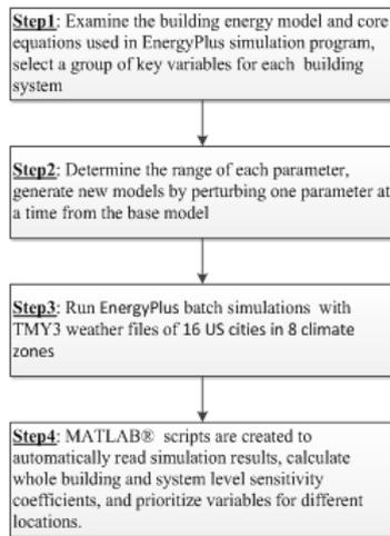
**Figure 2.** Procedure of conducting system level sensitivity analysis
