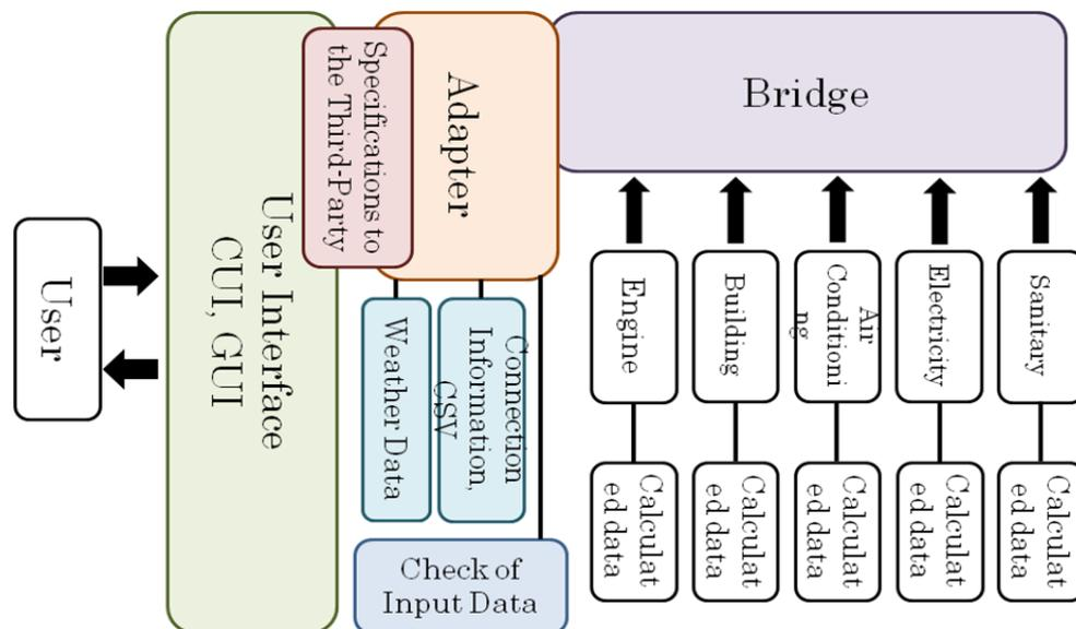
**Figure 7.** The outline of the whole configuration of an energy simulation tool viewed from UI
