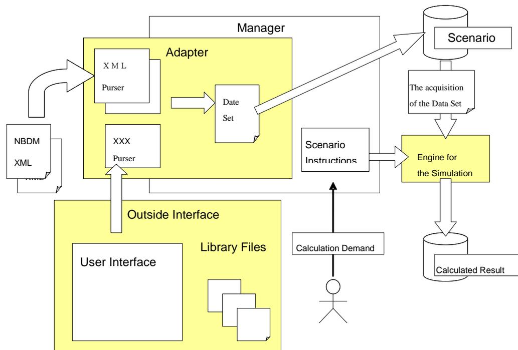
**Figure 6.** A brief data structure of the actually developed for MPC of HVAC system
