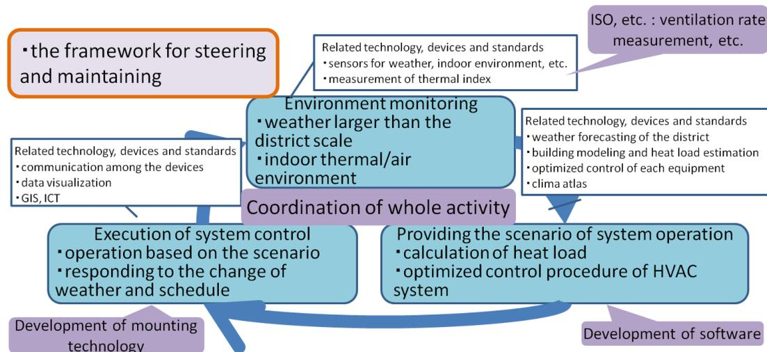
**Figure 1.** Concept of MPC for HVAC system
