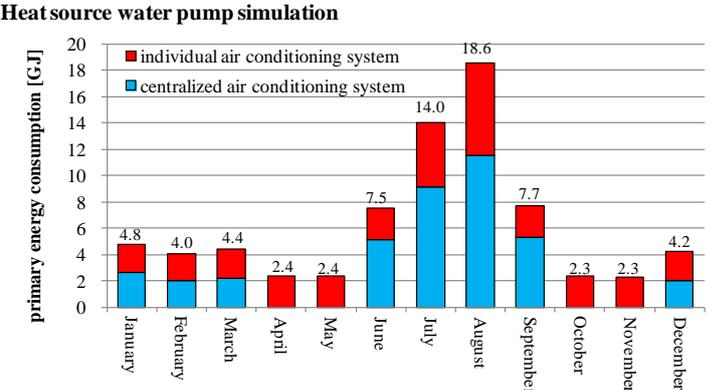
Figure 10. Monthly primary energy consumption of heat source water pump
