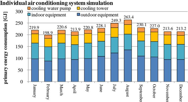
Figure 9. Total monthly primary energy consumption of individual air conditioning system
