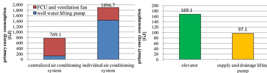
**Figure 11.** Primary energy consumption (left : well water lifting pump and fan (FCU and ventilation) / right : elevator and supply and drainage lifting pump)
