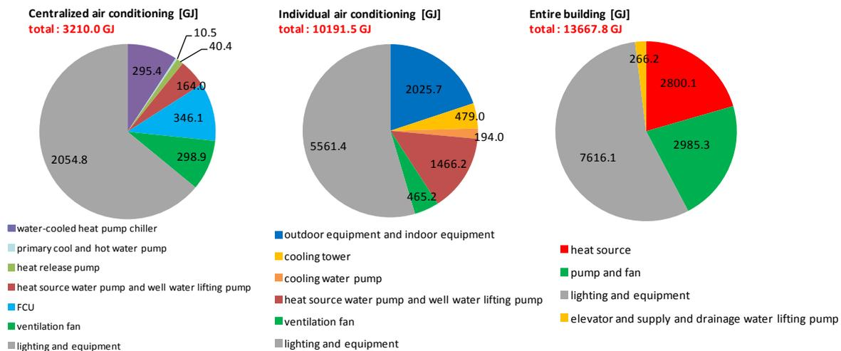
**Figure 13.** Annual primary energy consumption of centralized air conditioning system (left), individual air conditioning system (middle), and entire building (right)
