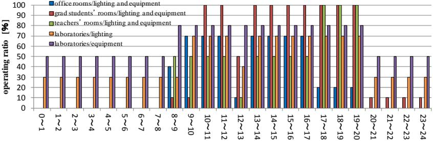
**Figure 4.** Design values of hourly operation ratio
