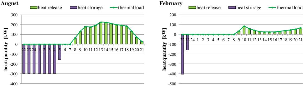
Figure 6. Hourly values of the heat storage (negative axis) and the heat release (positive axis) for a day in August (left) and February (right)
