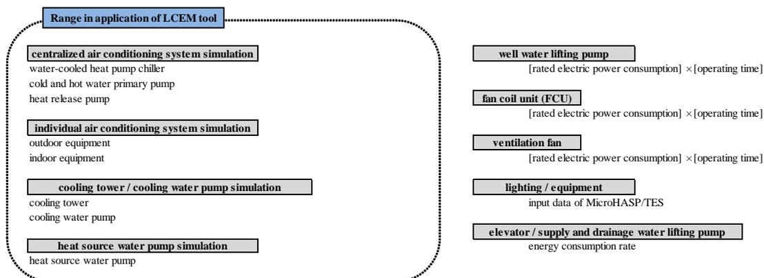
Figure 2. Application range of LCEM tool and calculation methods for energy consumption
