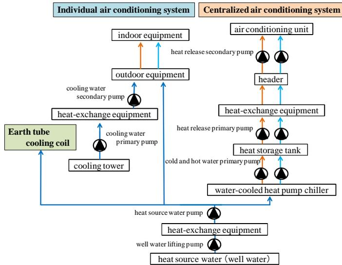
Figure 1. Heat source system diagram
