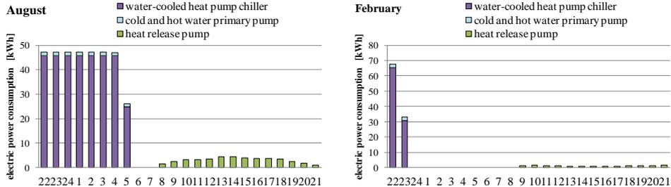
Figure 7. Electric power consumption in August (left) and February (right)
