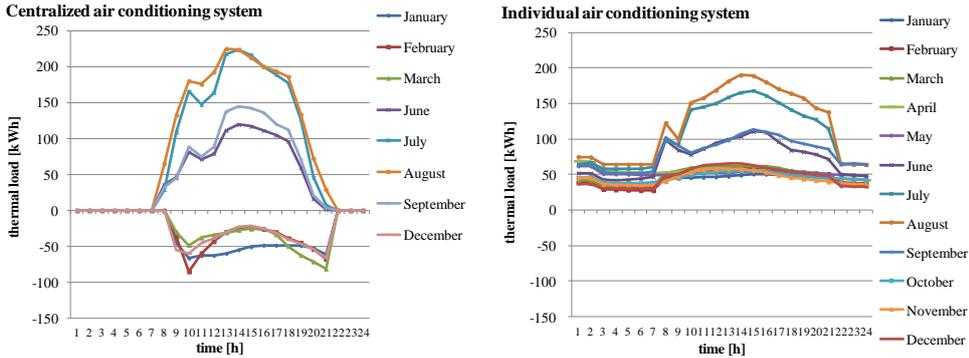
**Figure 3.** Cooling load (positive values) and heating load (negative values) on a representative day of each month for the centralized air conditioning system (left) and the individual air conditioning system (right)
