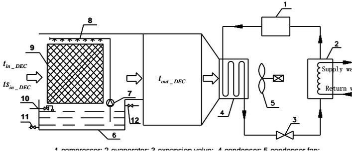
Figure 1. Schematic of EACC
