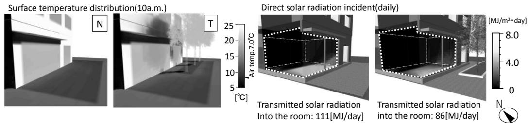
**Figure 4.** Distribution of surface temperature (10 a.m.) and incident daily direct solar radiation
