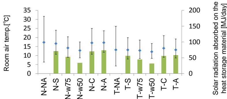
**Figure 5.** Daily fluctuation in room air temperature and solar radiation absorbed on the heat storage material
