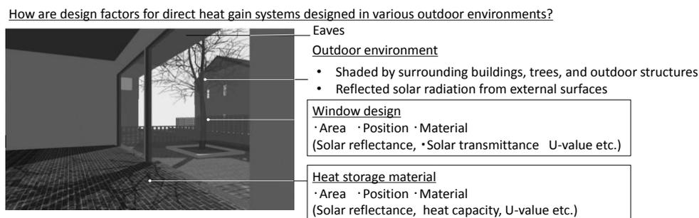
*Figure 1. Design factors for direct heat gain systems*
