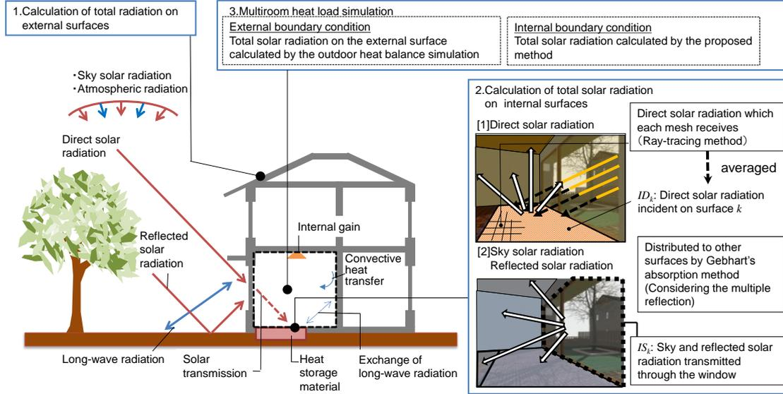
**Figure 2.** Outline of proposed simulation tool for predicting the performance of direct heat gain systems
