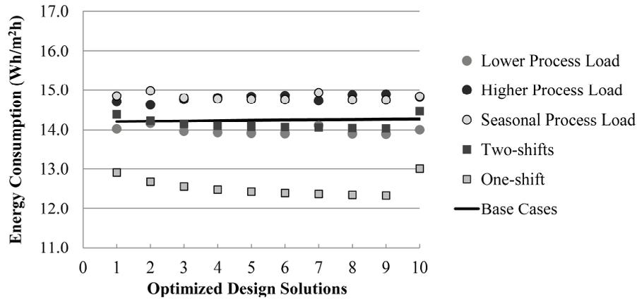
**Figure 2.** Energy consumption of optimized design solutions for the  $45W/m^2$  process load scenario with variations in process load and occupancy pattern.
