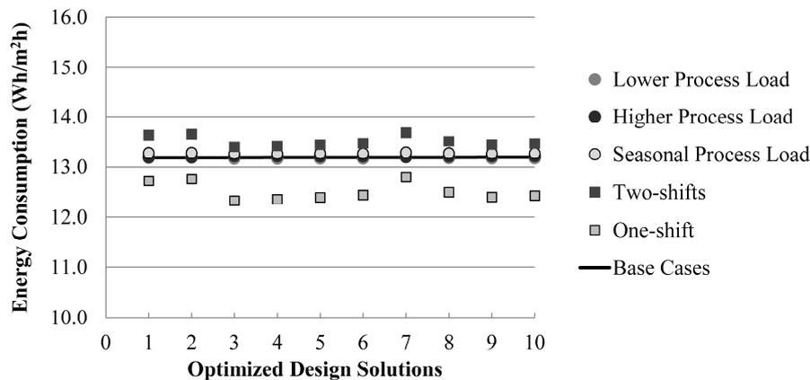
**Figure 1.** Energy consumption of optimized design solutions for the 5W/m<sup>2</sup> process load scenario with variations in process load and occupancy pattern.
