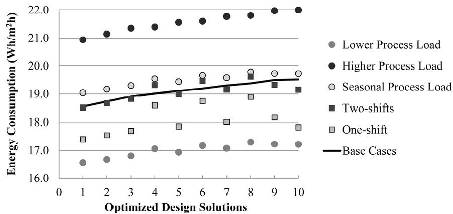
**Figure 3.** Energy consumption of optimized design solutions for the  $5W/m^2$  process load scenario with variations in process load and occupancy pattern.
