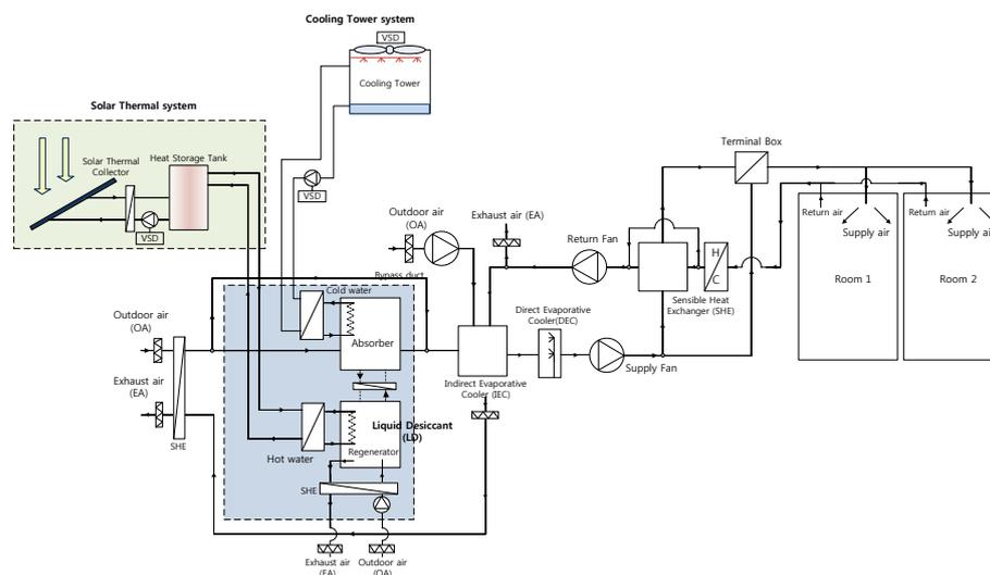
**Figure 2.** Solar thermal collector plant
