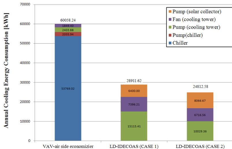
**Figure 3.** Comparison of annual cooling energy consumptions for different systems and CASEs
