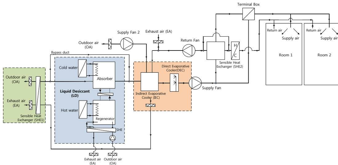
**Figure 1.** Schematic of desiccant and evaporative cooling assisted 100% outdoor air system
