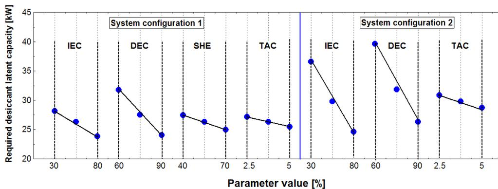
**Figure 2.** The influence of the effectiveness of components on the required latent cooling capacity
