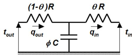
Figure 3: 2RIC wall model including two no dimensional parameters  $\theta$  and  $\phi$ .
