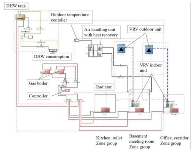
Figure 9: Circuit diagram for detailed HVAC system of the Hegyvidék office building
