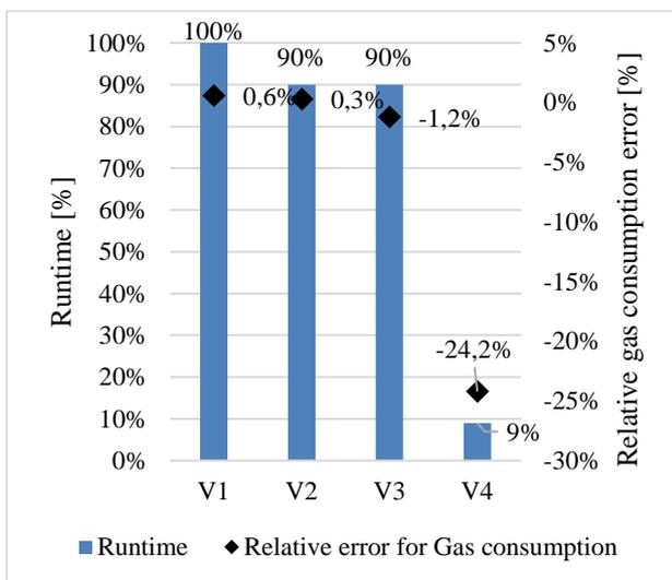
Figure 18: Simulation times of the model scenarios for the office building
