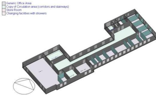
Figure 7: Zones of the ground floor with hanging partitions
