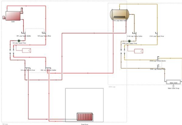
Figure 10: Circuit diagram for detailed HVAC system of the kindergarten
