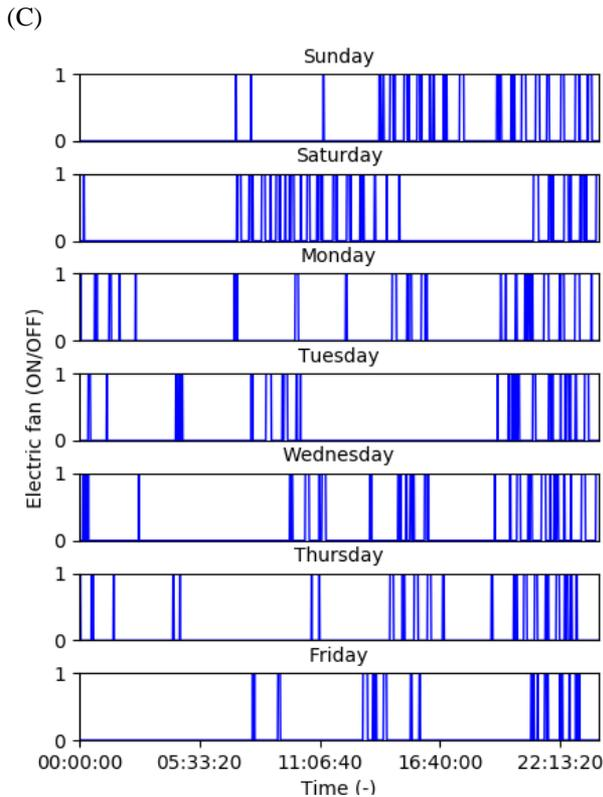
Figure 3: (A) Electricity consumption profile of 3-9 November 2018 for a household with A/C and electric fans for attaining thermal comfort; (B) A/C unit operation for retaining thermal comfort in the same household on 3-9 November 2018; (C) Electric fan operation in the same household on 3-9 November 2018.
