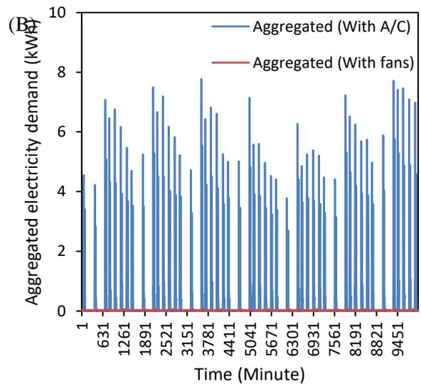
Figure 6: (A) Comparison of indoor operative temperature with and without A/C (with only fans) in a First floor flat: Bedroom and living; (B) Comparison of aggregated electricity demand with and without A/C in the building community for 3-9 November.
