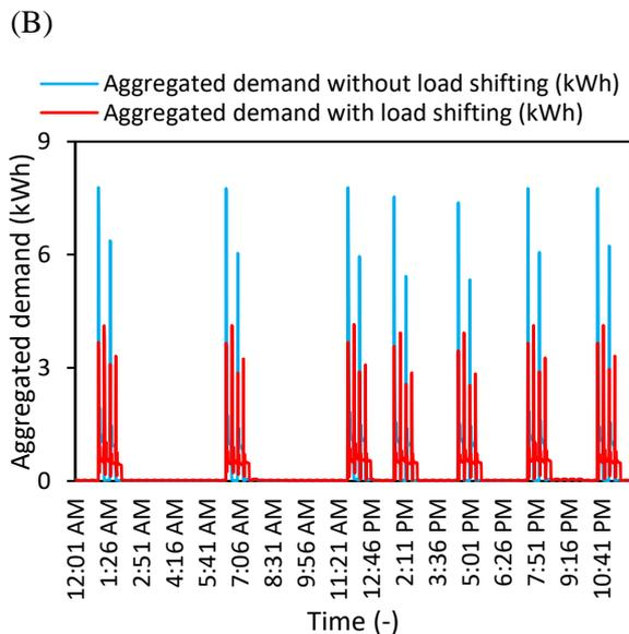
Figure 7: (A) Indoor and outdoor air temperature comparison; (B) Aggregated electricity demand with (red) and without 15-minute load shifting (blue) for 1 June in the building community.
