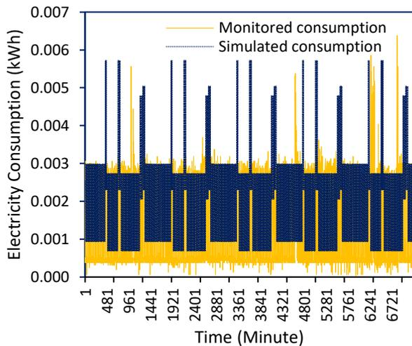
Figure 5: Minutely electricity consumption profile (monitored and simulated) for a household with fans to retain thermal comfort on 3-9 November 2018
