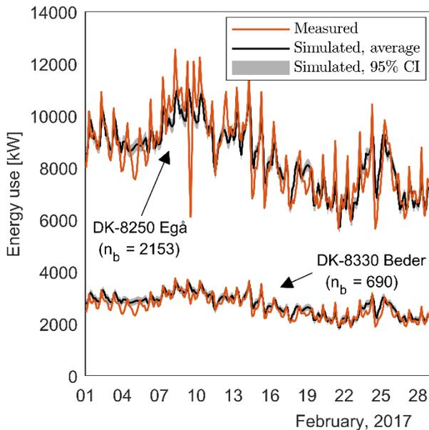
**Fig. 1.** Measured and simulated aggregated DH energy use (three-hourly) of two suburban towns, respectively. Simulated energy use consist of the 95% central posterior density region derived from aggregating 1000 random simulations from each of the individual building energy models. The average of the 1000 aggregated simulations is highlighted in black.
