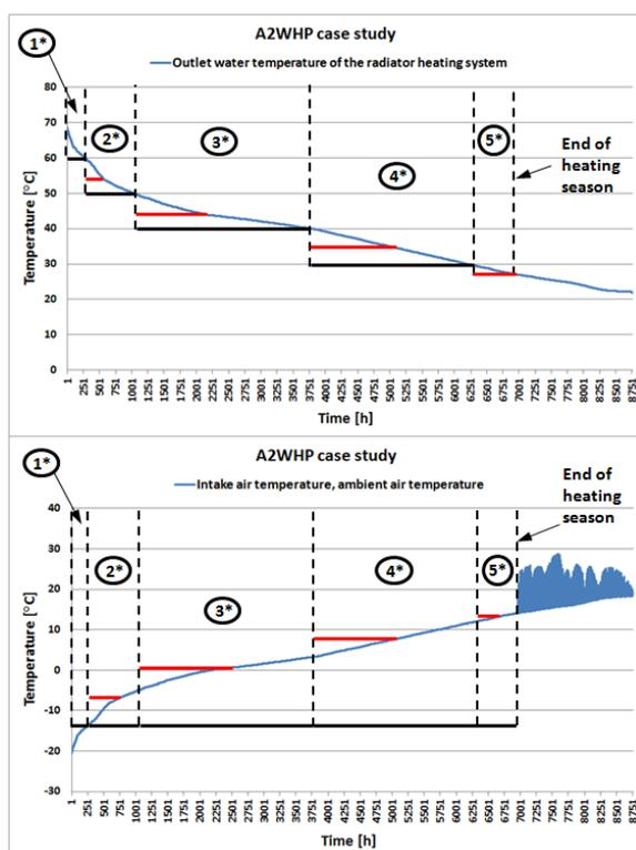
Figure 6 The temperature data of the heating system in the studied building and the ambient conditions for the detailed calibration of an A2WHP system
