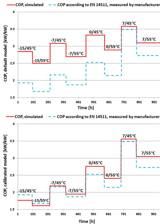
Figure 5 The performance of the simulated A2WHP system model, the default heat pump model (second from the bottom) and the calibrated heat pump model (bottom) according to 7/45 °C operating point presented
