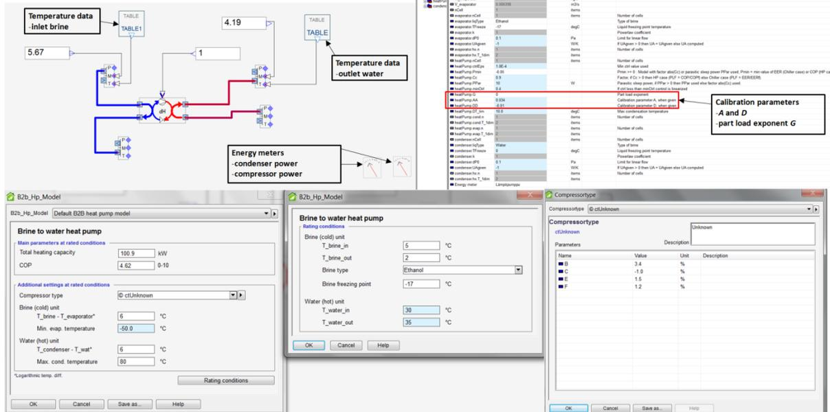
Figure 1 The calibration setup of the GSHP system model (top left), calibration parameters *A*, *D* and *G* (top right), calibration parameters *B*, *C*, *E* and *F* (bottom right), main parameters and settings at rated conditions (bottom left) and input data of rating conditions (bottom center)
