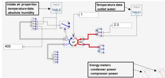
Figure 4 The calibration setup of the A2WHP system model
