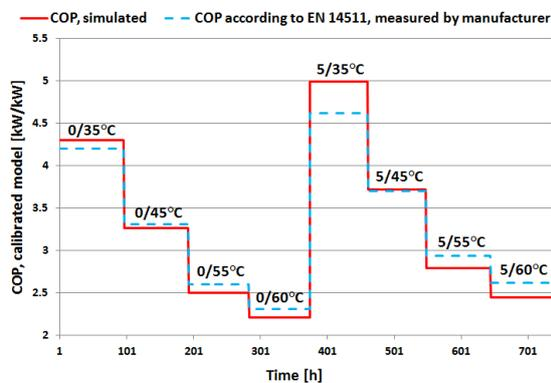
Figure 3 The energy performance of the simulated GSHP system model, calibrated heat pump model according to 5/45 °C operating point
