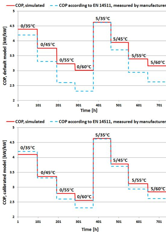
Figure 2 The performance of the simulated GSHP system model, the default heat pump model (second from the bottom) and the calibrated heat pump model (bottom) according to 5/35 °C operating point presented
