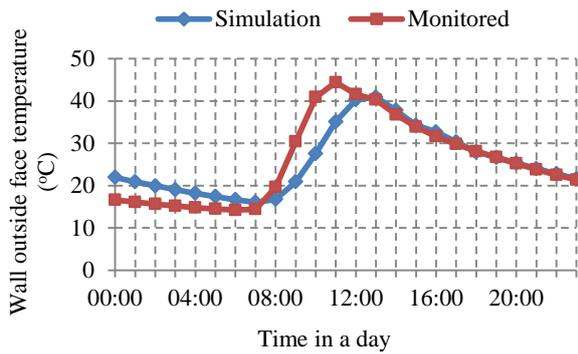
Figure 10 Trombe Wall outside surface temperatures
