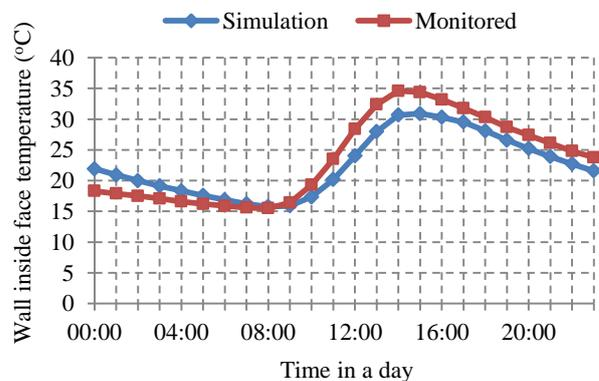
Figure 9 Trombe Wall inside surface temperatures
