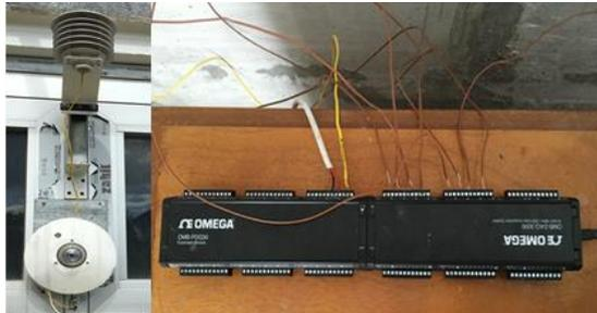
Figure 7 Close up view of the outdoor air thermocouple, pyranometer and data acquisition system
