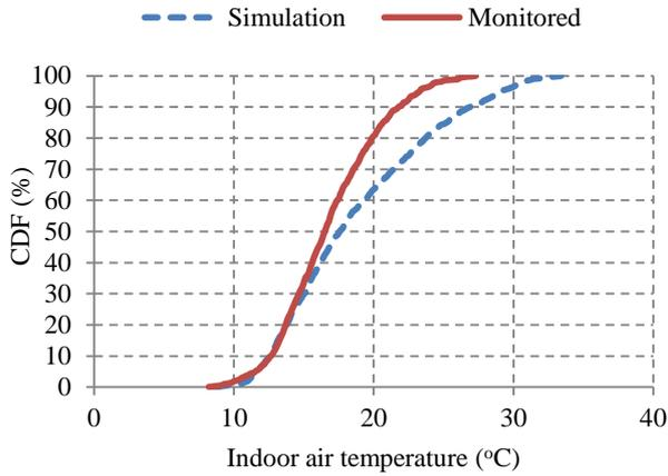
Figure 13 CDF curves for indoor air temperatures
