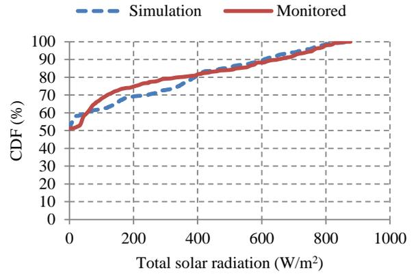
Figure 16 CDF curves for solar radiation values
