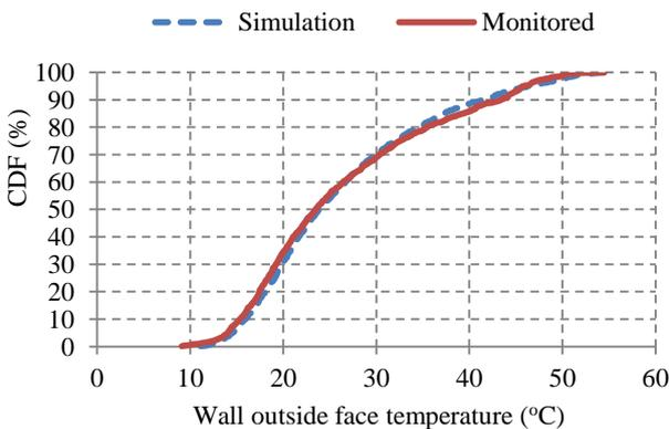
Figure 15 CDF curves for Trombe Wall outside surface temperatures
