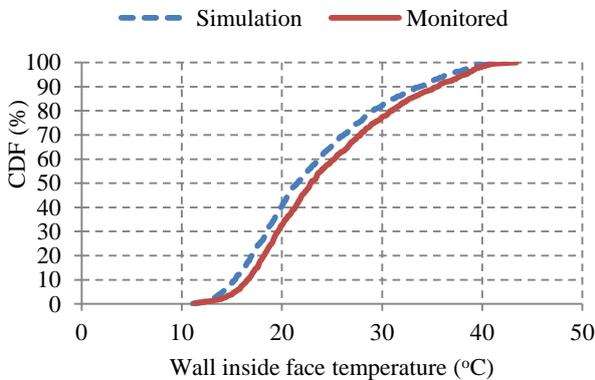
Figure 14 CDF curves for Trombe Wall inside surface temperatures
