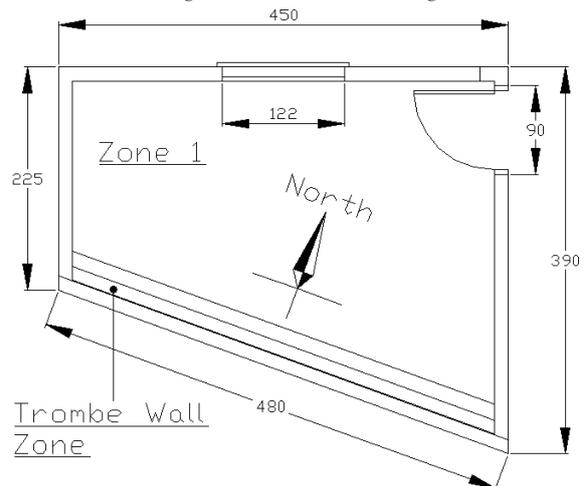
Figure 2 Plan of the test building (dimensions are in cm, thickness of the Trombe wall zone is 14 cm)
