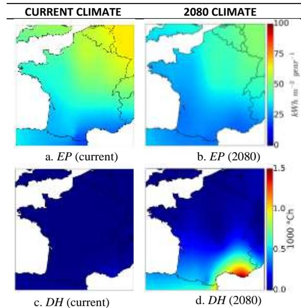
Figure 6 (a,b) energy demand ( $EP$ ) and (c,d) number of degree hour ( $DH$ ) of thermal discomfort for France for optimized solutions.
