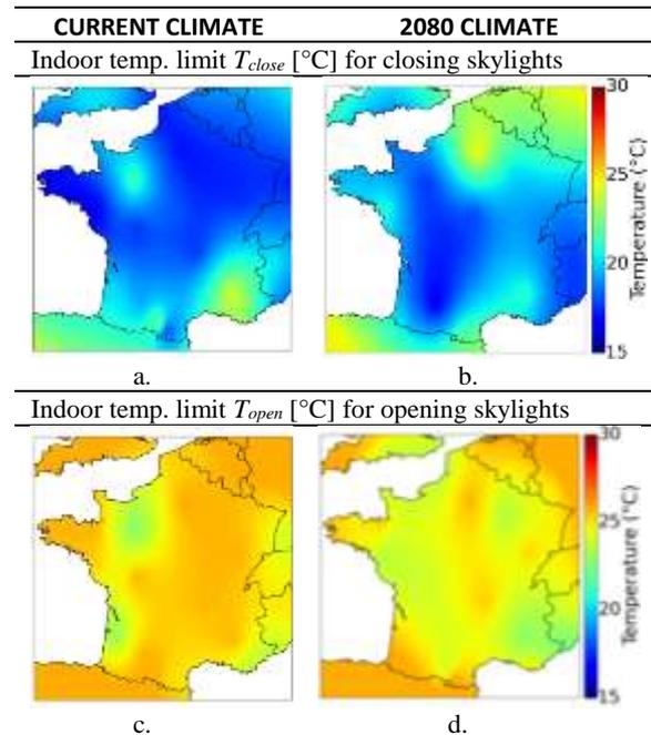
Figure 8 indoor air temperatures limits for skylights opening control for natural ventilation.
