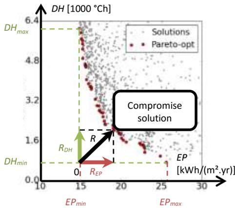
Figure 5 Pareto optimal solutions and compromise solution  $R$
