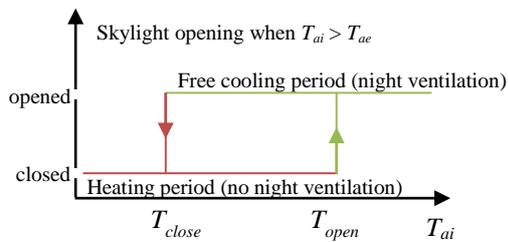
Figure 2 heating and free cooling periods determined by  $T_{close}$  and  $T_{open}$  parameters for night natural ventilation
