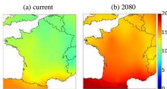
Figure 3 annual mean values of ambient temperatures ( $^{\circ}\text{C}$ ) for current (a) and future climate (b).
