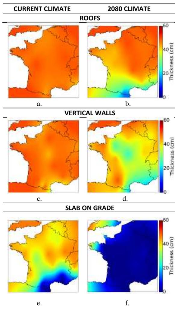
Figure 10 optimized thermal insulation thickness for walls.
