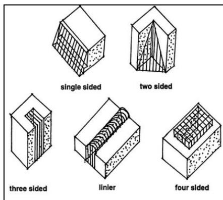
Figure 2: Five basic configurations of atria in buildings (Onyenobi, 2008)
