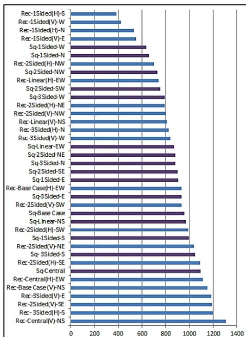
Figure 9: Rectangular and Square prototypes total annual heating and cooling loads (MWh)
