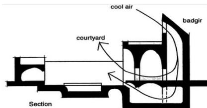
Figure 1: Section of a typical Persian house with courtyard and wind catcher in middle-east
