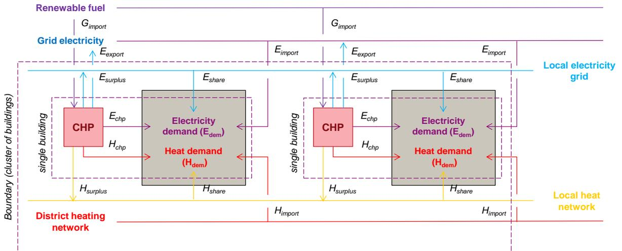
Figure 1: Energy flow in Case 3 (Energy transfer from surplus side to deficit side is allowed.)
