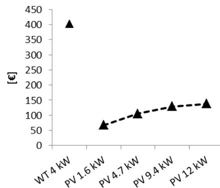
Figure 6 – The savings from reduced electricity import in the first year of operation, in Euro
