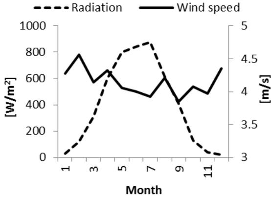
Figure 3 – The monthly averages for global radiation on the horizontal and wind speed in TRY12 (based on Kalamees et al., 2012)
