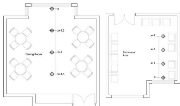
Figure 4 Plan view: measurement points in dining room (left) and communal area (right). Source: author’s diagram
