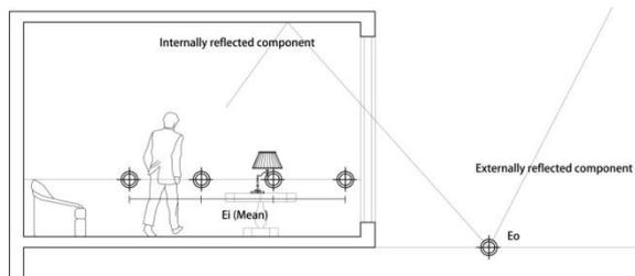
Figure 6 Daylight factor. Source: author's diagram
