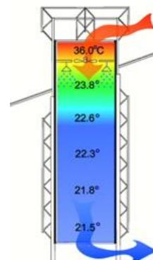
Figure 1- PDEC Airflow and Temperature Process (Ben-Gurion University of Negev, 2016)
