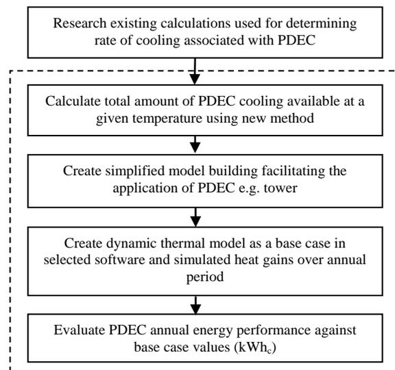
*Figure 2 PDEC Design Flow Diagram*
