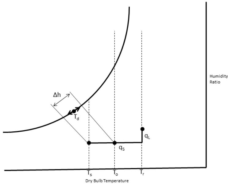
**Figure 5** Allowable variation in apparatus dewpoint temperature for the cool, dry outdoor air condition
