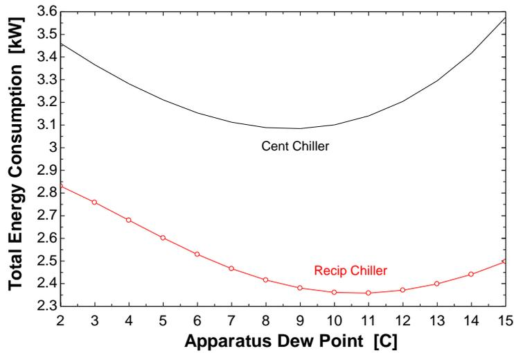
**Figure 7** The variation in total system energy input with chilled water temperature for both chillers for VAV system in cool & dry condition
