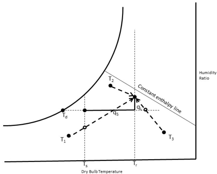
**Figure 6** Operating logic considerations for energy recovery control
