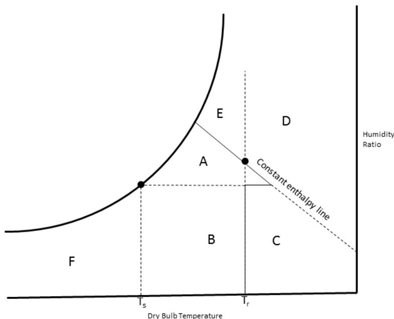
**Figure 1** Typical logic for economizer control
