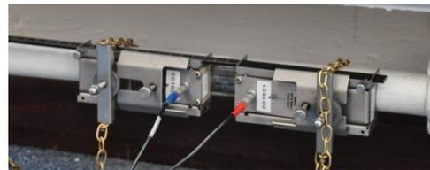
Figure 4 Transducer mounting.
