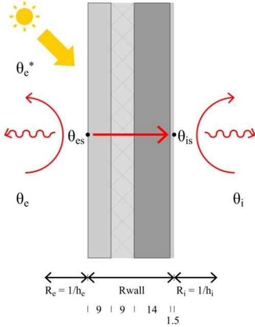
Figure 2 – Wall properties and assumed heat transfer mechanisms.
