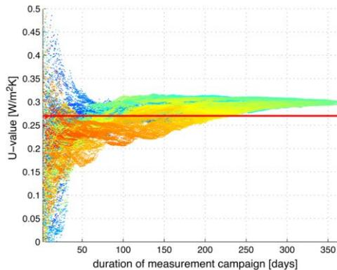
Figure 4 – U-value estimation through multiple regressions applied on measurement campaign data with different starting dates and duration based on simulations over the course of one year. The data points are coloured according to the average  $Q$  over the course of the measurement campaign: red points indicate a high average  $Q$ , blue points indicate a low average  $Q$ .
