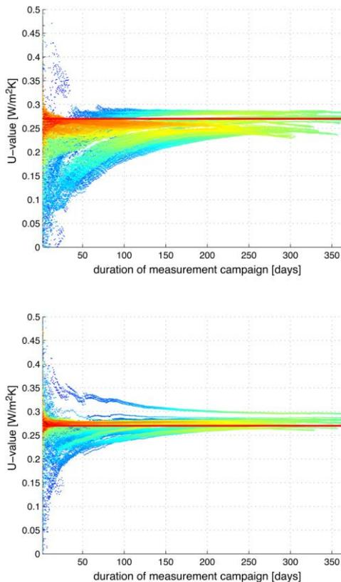
Figure 6 – U-value estimation through linear regressions assuming a transformed equation applied on measurement campaign data with different starting dates and duration based on simulations over the course of one year. Top: basic regression; bottom: thermal lag ( $\Delta T$  and  $S$ ) taken into account. The data points are coloured according to the average  $Q$  over the course of the measurement campaign: red points indicate a high average  $Q$ , blue points indicate a low average  $Q$ .
