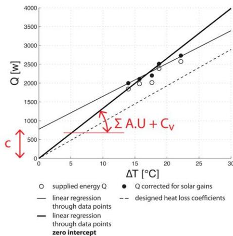
Figure 1 – Illustration of a simple linear regression assuming fictive co-heating measurement data, corrected for solar gains.
