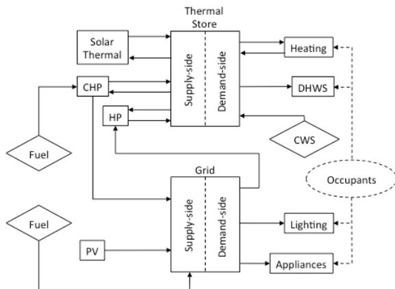
**Figure 2, Block schema of the heat and electricity generation, storage and demand system.**
