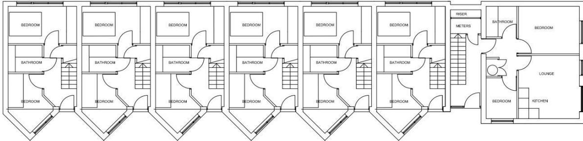
**Figure 1, the ground floor plan of the building. The upper floors to the 6 identical flats are an open plan living space with kitchen. The flat to the right is the first storey of three identical units. The building dimensions are approximately 36m by 8m and 9 m at the highest point.**
