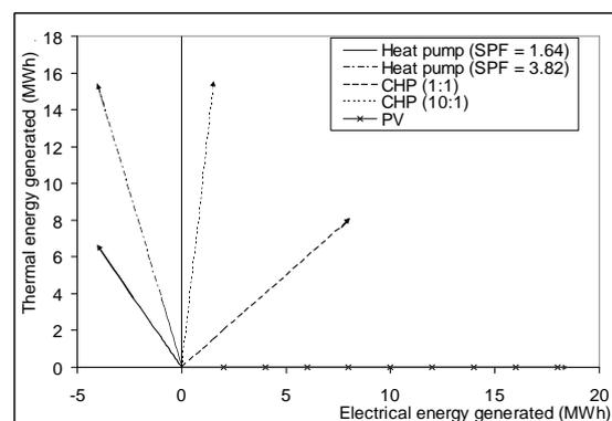
Figure 5 thermal generation as a function of electrical power consumption/production with different type of generation plant.
