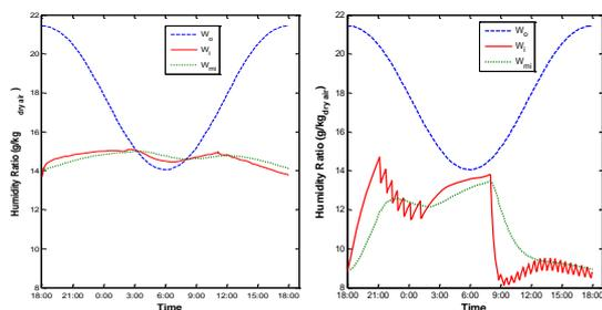
Figure 4 Comparison of daily humidity ratio profiles (l) optimized operation (r) conventional operation
