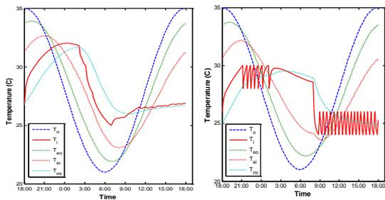
Figure 3 Comparison of daily temperature profiles (l) optimized operation (r) conventional operation
