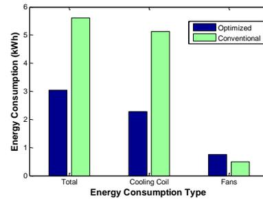
Figure 1 Energy consumptions of the optimized and conventional operations
