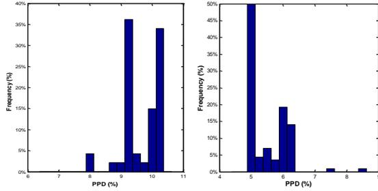
Figure 6 Comparison of daily PPD distributions during office hours (l) optimized operation (r) conventional operation
