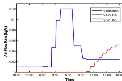
Figure 2 Dynamic profiles of air flow rates in the optimized operation strategy
