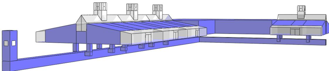
*(c) A whole building concept option (single air supply culvert)*
