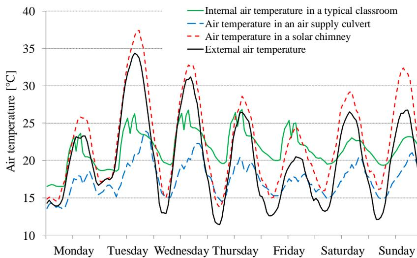
Figure 6 Example air temperatures in the natural ventilation system during a hot period (31<sup>st</sup> May to 6<sup>th</sup> June)
