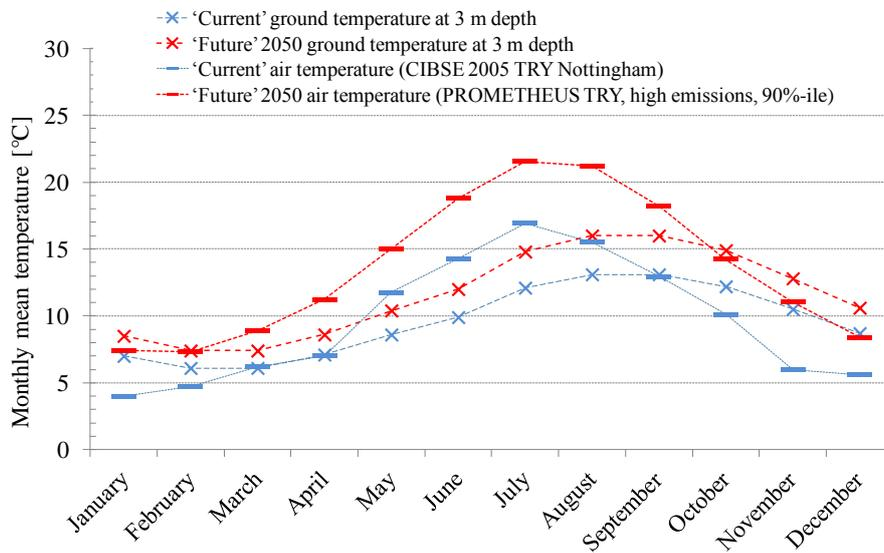
Figure 5 Monthly mean air- and ground temperature at 3 m depth for the current and future climates
