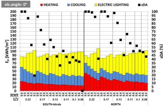
Fig. 4 – Global primary energy demand and sDA<sub>300/50%</sub> values for all room configurations with  $\gamma=0^\circ$ .
