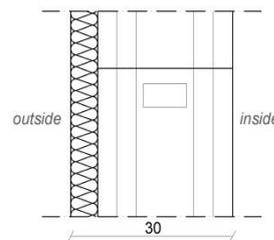
Fig. 4 – Section of wall made of *Gasbeton* blocks
