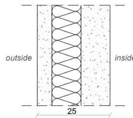
Fig. 3 – Section of wall with precast concrete panels
