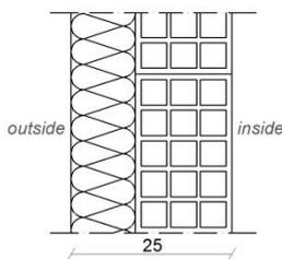
Fig. 2 – Section of hollow bricks wall with external insulation layer
