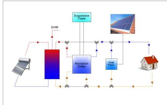
Fig. 11 – Summer functional scheme of the plant
