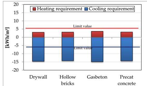
Fig. 6 – Building energy consumption in function of the different opaque walls
