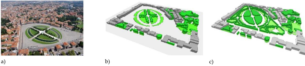
Figure 1 – The area (a) and the model area in ENVI-met used for the simulations of the “AsIs” scenario (b) and the “Green ground” scenario (c)
