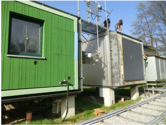
Fig. 5 – PASSSYS test cell at UIBK with installed functional models, left cell: 1st functional model (MVHR next to window), right cell: 2nd functional model ( \mu HP and MVHR) – photo: UIBK
