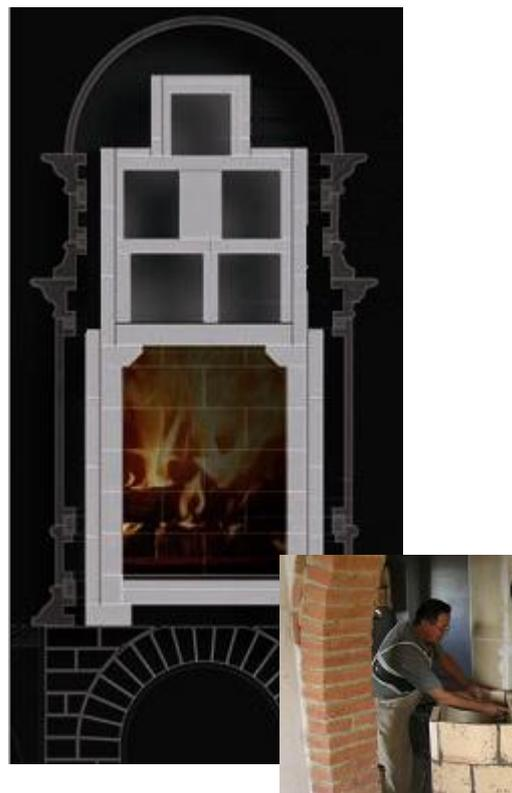
Fig. 1 – View of a project design of a modern stove, where the combustion chamber and twisted conduit are visible and a phase of its construction (Barberi Ltd).
