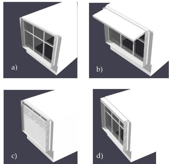
Fig. 4 – DAYSIM geometry, a) office room b) overhang c) deployed external blinds, d) retracted external blinds
