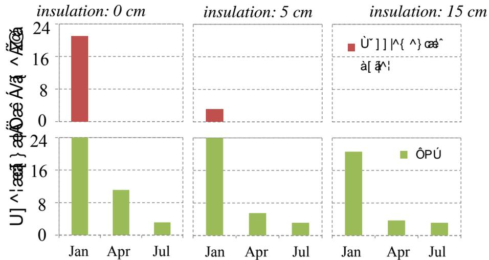
Fig. 7 – Operational time for a 30 kW<sub>el</sub> (80 kW<sub>th</sub>) power plant. Three average days (January, April, July) are considered for different building configurations. Supplementary boiler is supposed to be 80 kW<sub>th</sub>
