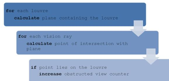
Fig. 4 – Outline of routine used to calculate obstructed view
