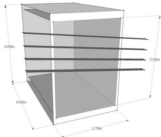
Fig. 1 – Overview of the thermal model
