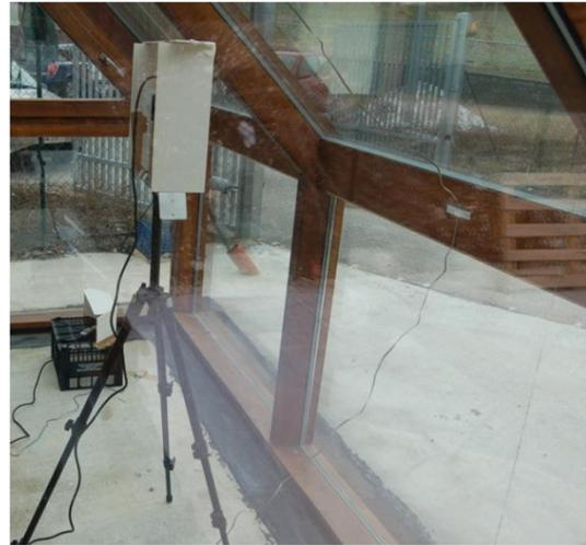
Fig. 1 – Sensors in the sunspace prototype during a monitoring campaign
