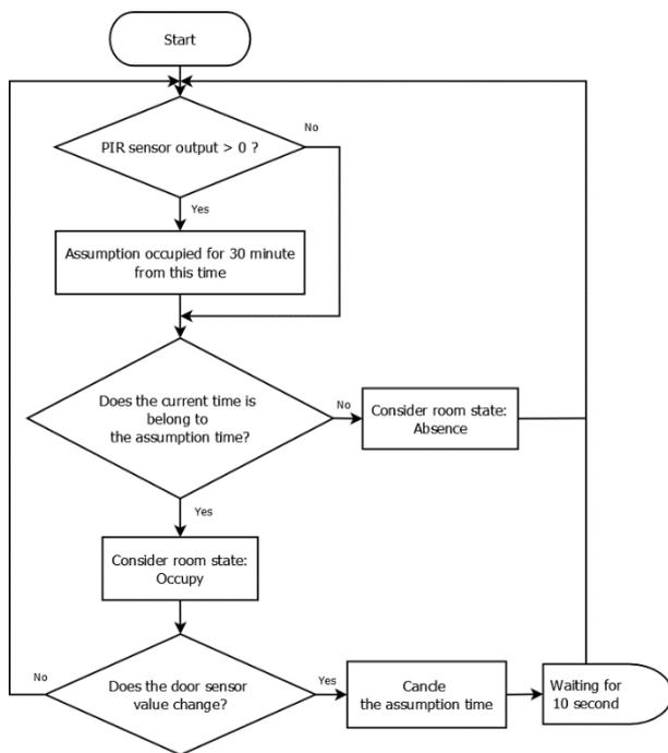
Figure 10. The flow chart of an occupancy detection algorithm
