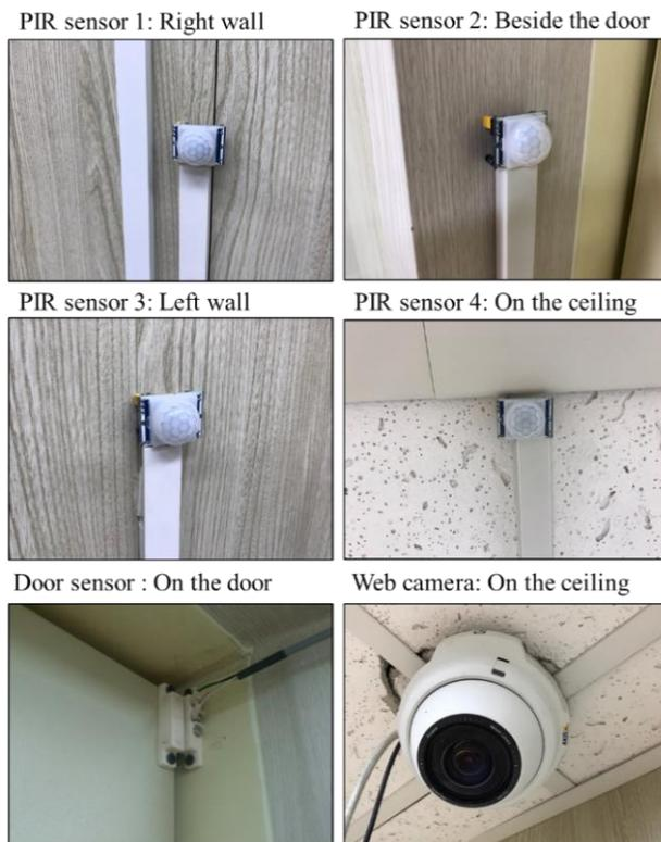
Figure 2. The appearance of PIR, door sensor and Web camera
