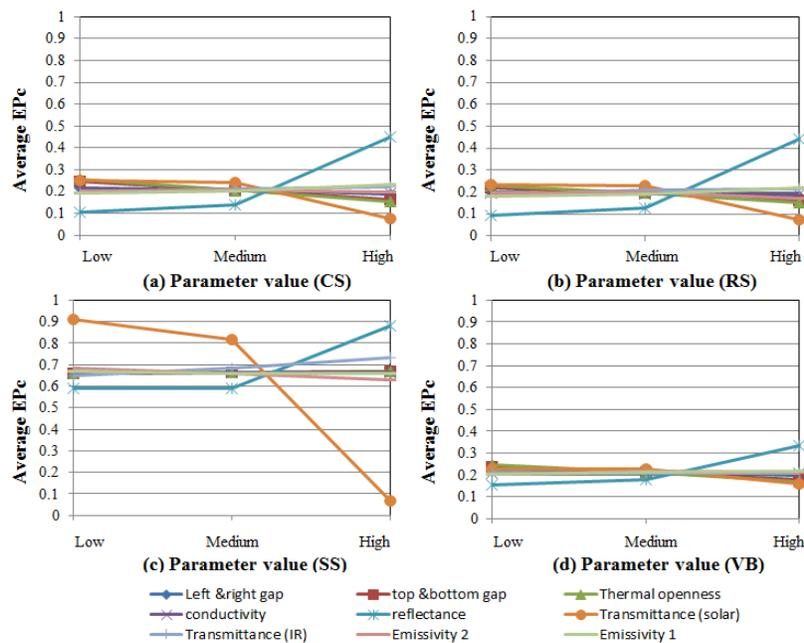
Figure 3: Impacts of different parameters on annual cooling energy performance in Houston; (a) interior cellular shades, (b) interior roller shades, (c) exterior solar screens, (d) interior venetian blinds
