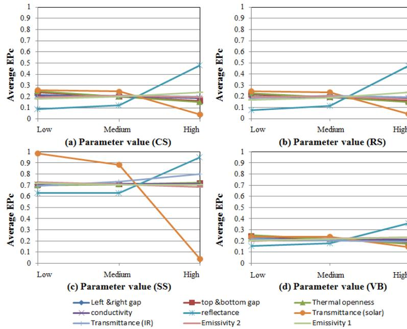
Figure 4: Impacts of different parameters on annual cooling energy performance in Washington, DC; (a) interior cellular shades, (b) interior roller shades, (c) exterior solar screens, (d) interior venetian blinds
