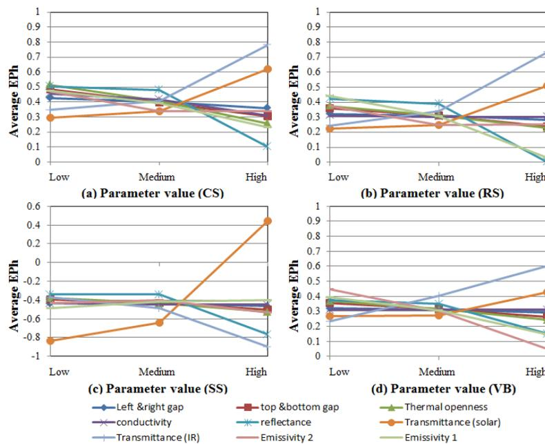
Figure 5: Impacts of different parameters on annual heating energy performance in Washington, DC; (a) interior cellular shades, (b) interior roller shades, (c) exterior solar screens, (d) interior venetian blinds
