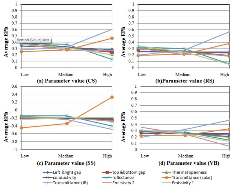
Figure 6: Impacts of different parameters on annual heating energy performance in Minneapolis; (a) interior cellular shades, (b) interior roller shades, (c) exterior solar screens, (d) interior venetian blinds
