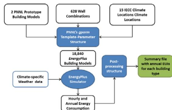
Figure 4: Block Diagram of the Simulation Process
