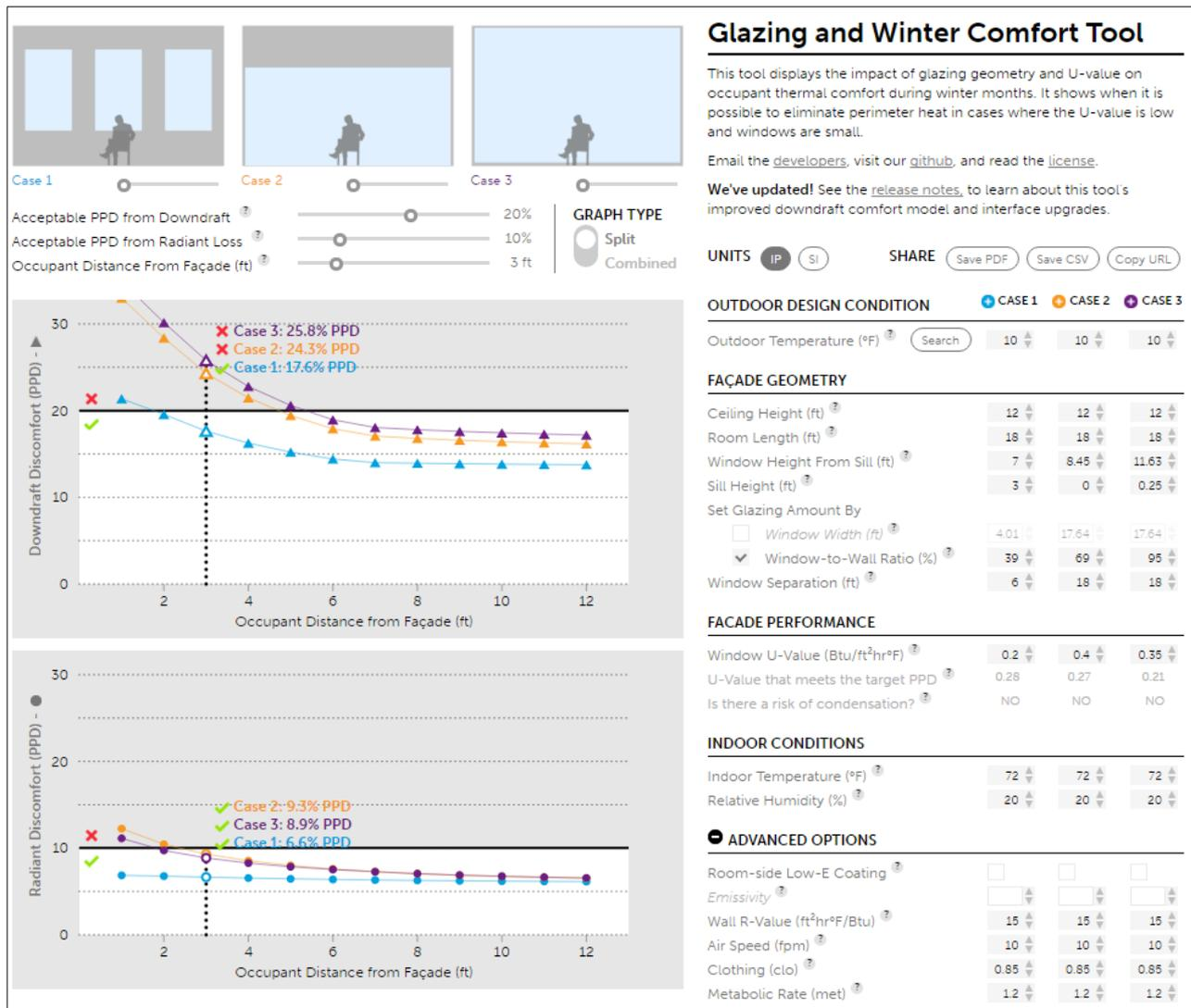
Figure 1. Thermal and Winter Comfort Tool Interface
