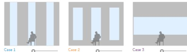
Figure 4. Three glazing scenarios with 40% window-to-wall ratio
