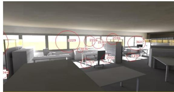
Figure 7: Luminance distribution for a critical hour.
