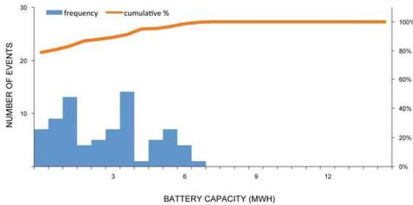
Figure 7: Approximate Battery Capacity (MWh) Requirements for 72-hr Event (Suite of Improvements with Reduced Operation and Additional PVs)
