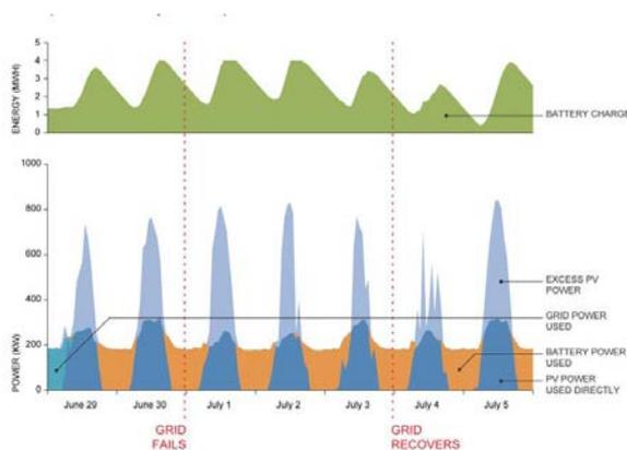
Figure 5: Facility Performance for Example of 72-hr Event- December (4MWh Battery + Suite of improvements).
