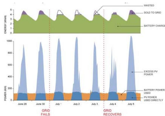
Figure 9: Facility Performance with reduced operation for Example of 72-hr Event- June (4MWh Battery + Suite of improvements+ Extra PVs+ Load Shedding).
