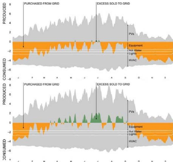
Figure 2: Annual Net Zero Energy Profile (MWh/day, weekly average) in two different design alternatives: with a suite of improvements (top graph) and with the suite of improvements and additional PVs (bottom graph).
