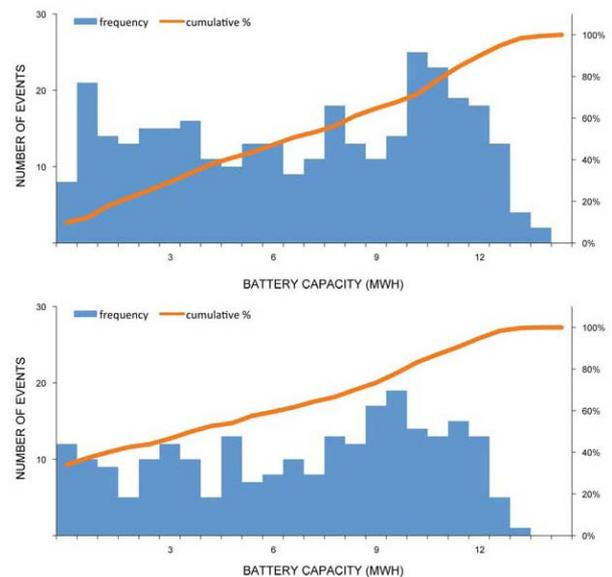
Figure 4: Battery Capacity (MWh) Requirements for 72-hr Events during normal operation in the suite with normal operation (top) and the suite with additional PVs (bottom).
