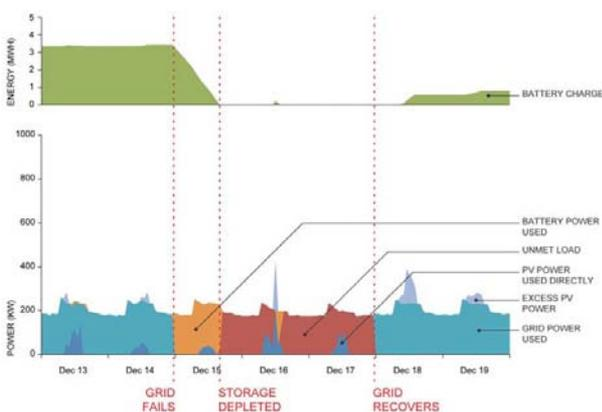
Figure 6: Facility Performance for Example of 72-hr Event- June (4MWh Battery + Suite of improvements).
