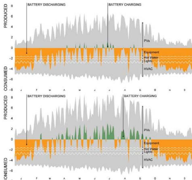
Figure 3: Annual 72-Hour Energy Performance (MWh/day, 3-day average) in two different design alternatives: with improvements (top graph), and with the suite of improvements and additional PVs (bottom graph).
