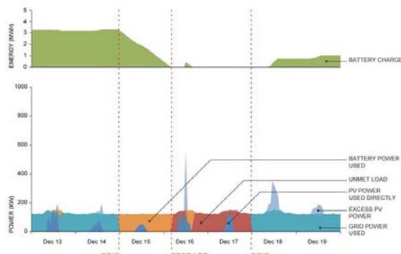
Figure 8: Facility Performance with reduced operation for Example of 72-hr Event- December (4MWh Battery + Suite of improvements+ Extra PVs+ Load Shedding).
