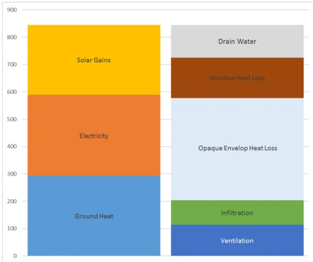
Figure 11: Energy balance of a simulation model
