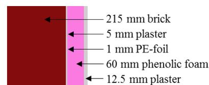
Figure 2: Internally insulated solid wall – construction assembly (external to internal)
