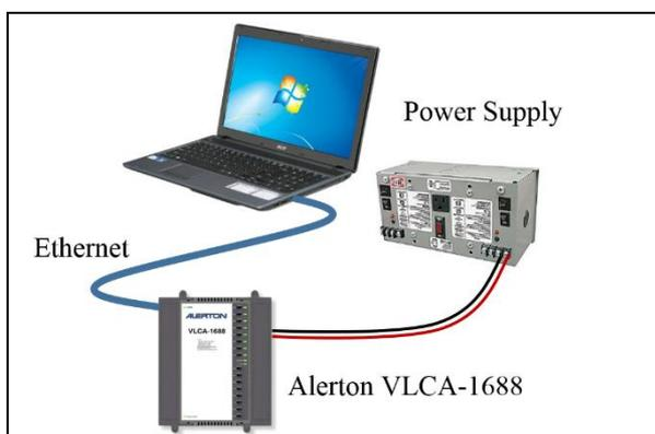
Figure 3: Alerton controller to energy model set-up
