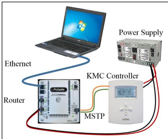
Figure 2: KMC controller to energy model set-up
